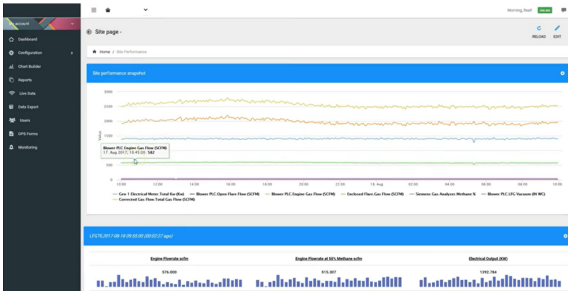
View of Sanborn Head's proprietary Landfill Gas Management Suite™ software that allows for remote monitoring of landfill gas collection and control systems while simplifying data management and reporting.
