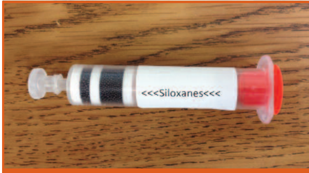
Figure 1. Sorbent Tube Filled with Solid Adsorbent Media for Sampling Siloxanes in LFG.
